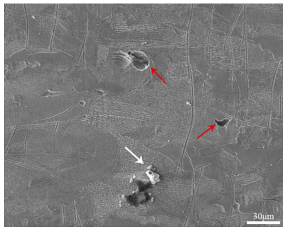
Figure 5. Microstructural defects of the stent.
