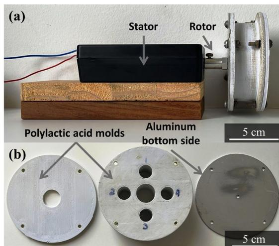
**Figure 1.** System used for freezing step while the slurry was in constant rotation: (a) side view of the system, and (b) poly(lactic acid) mold and the aluminum base plate.
