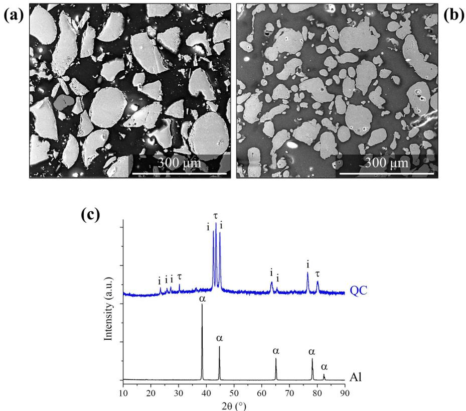
**Figure 2.** SEI micrographs of (a) QC and (b) Al particles, and (c) XRD patterns of these powders.
