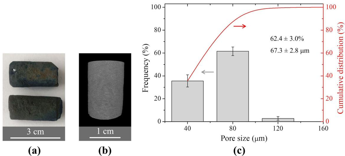
**Figure 3.** (a) Digital photograph of the samples produced, (b) 3D micro-CT image of an obtained scaffold, and (c) Pore size distribution evaluated by micro-CT for the scaffolds prepared in this study.
