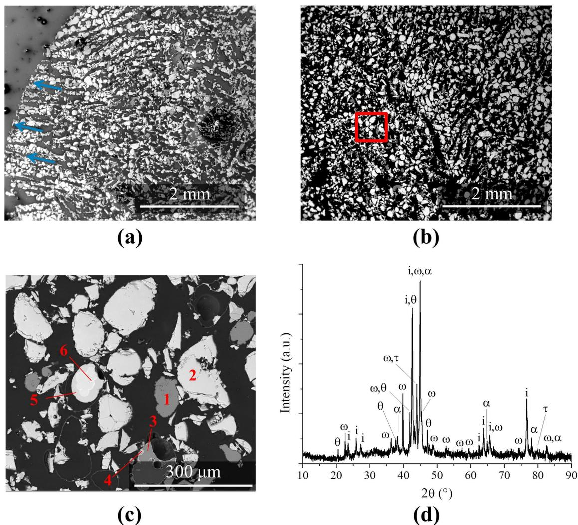
**Figure 4.** (a) Cross-sectional and (b) longitudinal SE images, (c) BE image of the region highlighted in (b), and (d) a typical XRD pattern taken for the prepared scaffolds.
