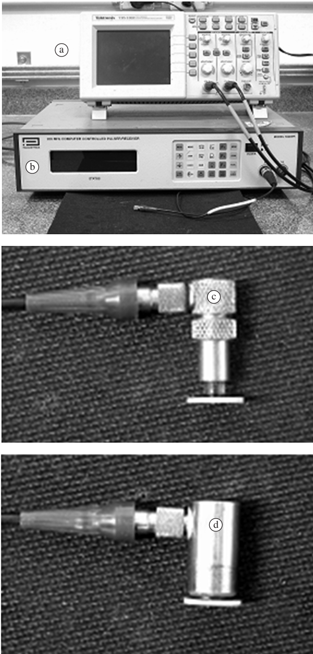
Figure 1. Images of a) oscilloscope, b) ultrasonic pulser-receiver, c) longitudinal wave transducer, and d) shear wave transducer used to measure sonic velocities. In c,d), a disk-shaped specimen in contact with the transducer is also shown.
