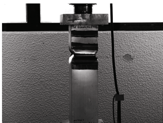
Figure 12. Initial plastic fold formed in geometry 4laser-p2.
