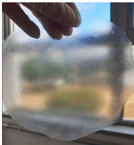
Figure 2. CMC film with EO rue for transparency and opacity evaluation. Source: Authors.
