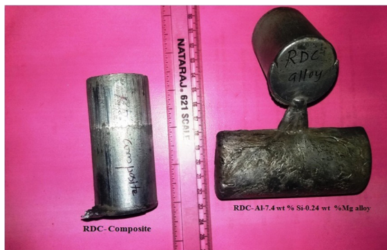
Figure 1. Rheo-Die- Cast (RDC) Al-Si-Mg alloy and composite samples
