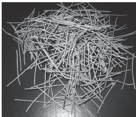
Figure 1. Cut waste steel wires.
