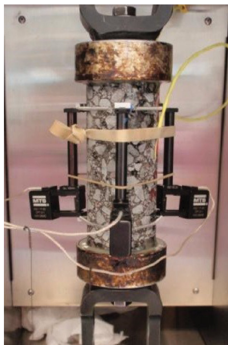
Figure 4. Instrumented sample in temperature chamber.
