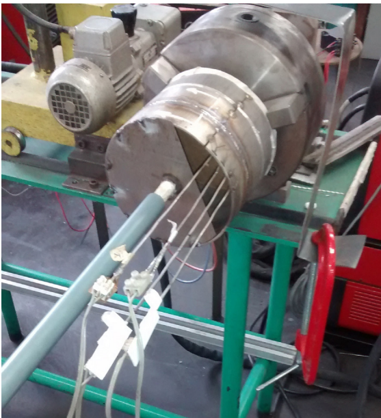
Figure 1. Experimental welding of UNS S32750 SDSS tube (two overlapping autogenous welding pass were carried out: clockwise and counterclockwise).
