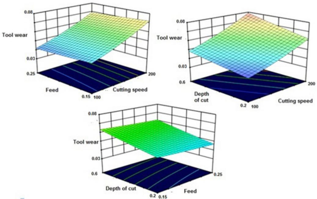
Figure 5. Effect of tool wear with a) cutting speed and feed b) cutting speed and depth of cut c) feed and depth of cut.
