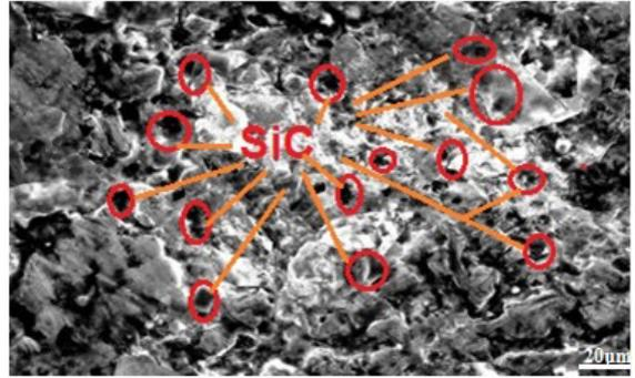
Figure 1. Microstructure of AA7075 with 15 wt % SiC.
