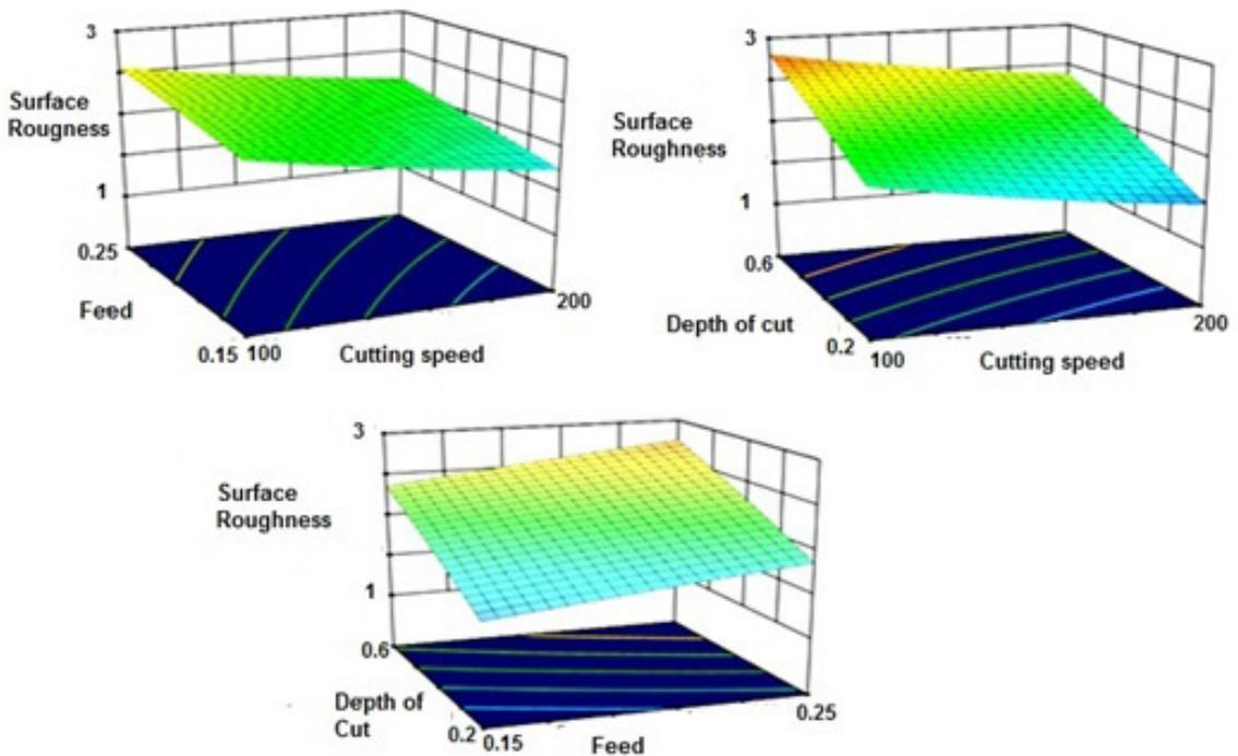
Figure 6. a) Effect of surface roughness with a) cutting speed and feed b) cutting speed and depth of cut c) feed and depth of cut.
