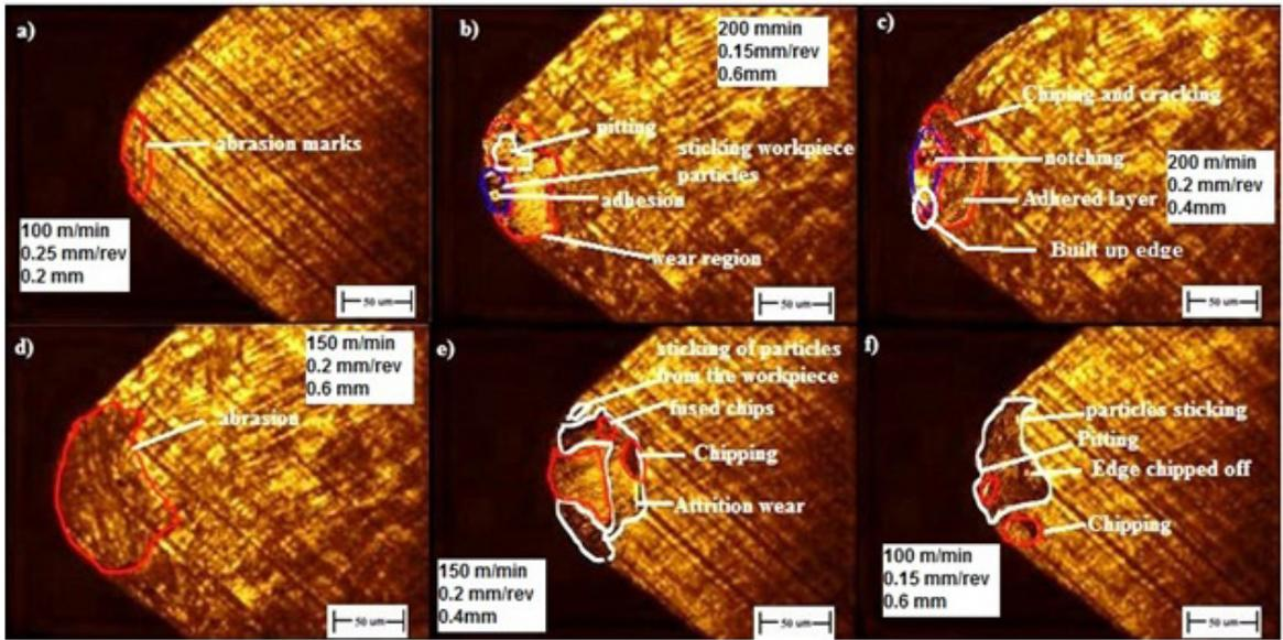
Figure 9. wear formation on cutting tool under different cutting speed, feed and depth of cut.
