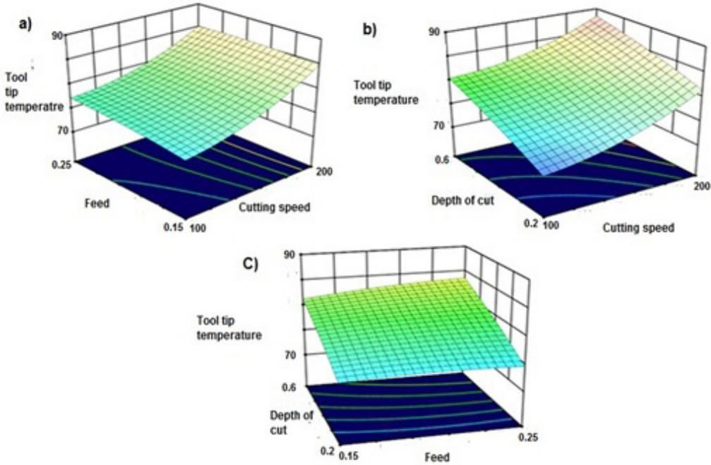
Figure 4. Effect of tool tip temperature with a) cutting speed and feed b) cutting speed and depth of cut c) feed and depth of cut.
