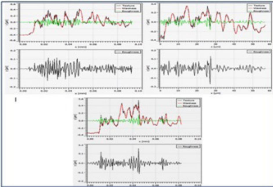
Figure 11. Surface profile graph at different cutting speed.
