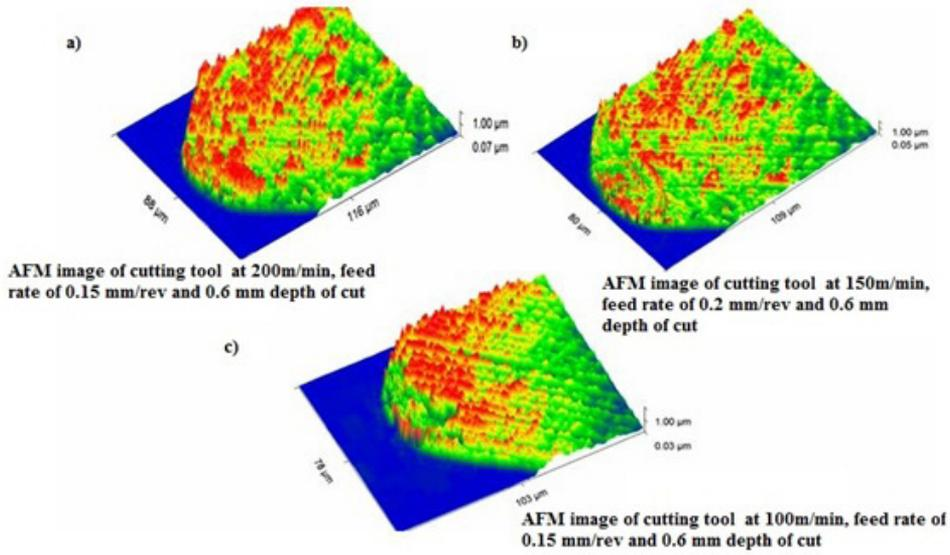
Figure 10. Tool surface morphology at different cutting speed.
