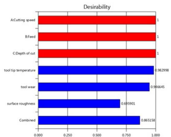
**Figure 8.** Bar graph of desirability of multi objective function.
