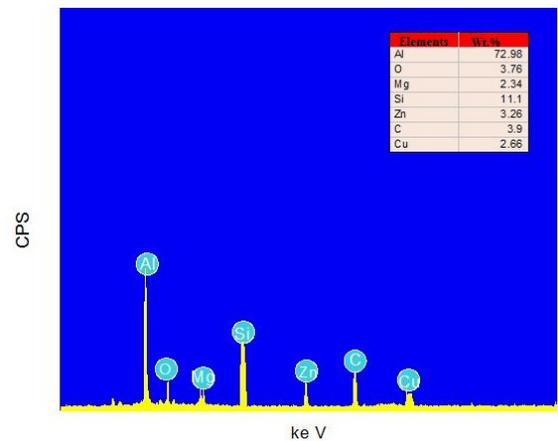
Figure 2. Energy dispersive X-Ray (EDX) profile of AA7075 with 15 wt % SiC.
