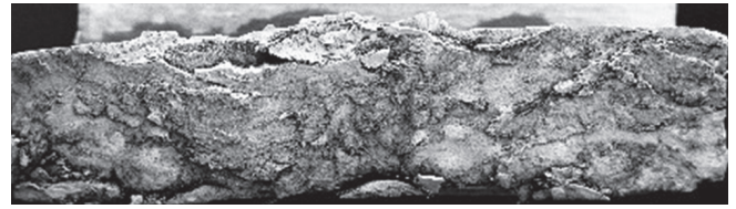
Figure 7. Cross-sectional view at the fracture surface of compression failed test coupon
