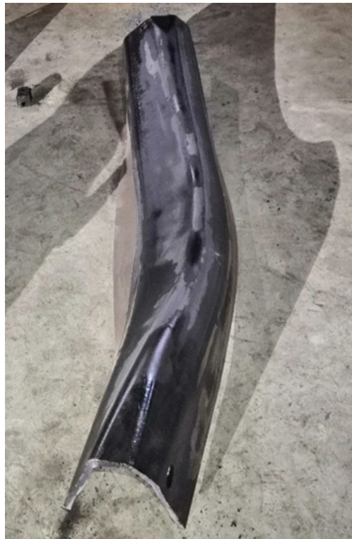
Figure 15. The trial hot forming process of the V-shaped part: (a) pressing process and (b) after unloading.
