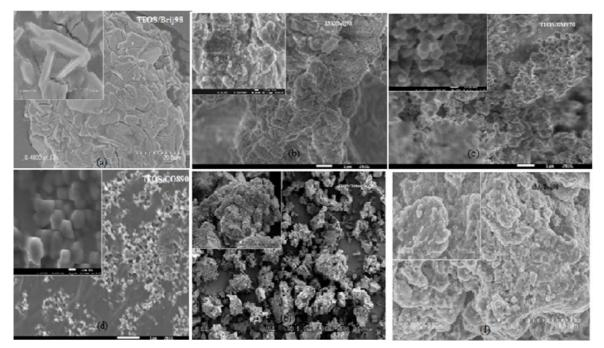
Figure 2. Scanning electron micrographs (SEM) of: TEOS/Brij98 and 13X/Brij98 (top); TEOS/DM-970 and TEOS/CO-890 (bottom).
