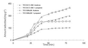
Figure 4. Adsorption breakthrough curves of acetone and 1-propanol over TEOS/CO-890 and TEOS/Brij98
