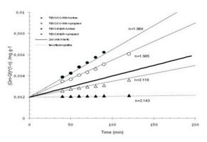
Figure 6. Acetone and 1-propanol kinetics adsorption onto purely silica at 298K (solid points: experimental; dashed lines: model)
