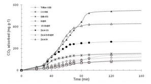
Figure 5. Adsorption breakthrough curves of CO2 over TEOS/ CO-890; TEOS/DM-970; TEOS/Brij98; 13X/Brij98; TEOS/ Triton-X-100; 3A/Brij98; Zeol-13X and Zeol-3A.
