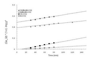
**Figure 7.** Carbon dioxide kinetics adsorption onto purely silica at 298K (solid points: experimental; dashed lines: model)
