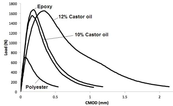
**Figure 3.** Typical Load vs. CMOD of castor oil and synthetic polymer mortars.
