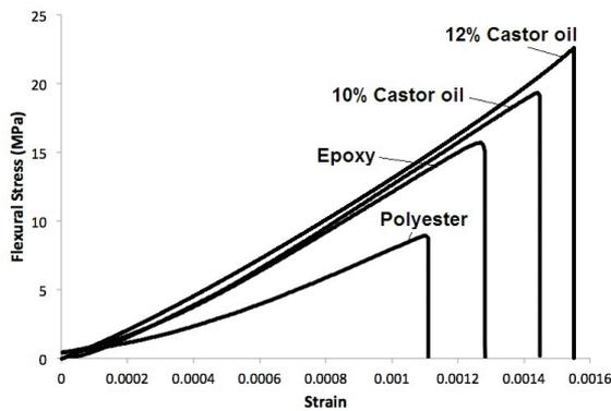
**Figure 2.** Typical flexural stress vs. strain of castor oil and synthetic polymer mortars.
