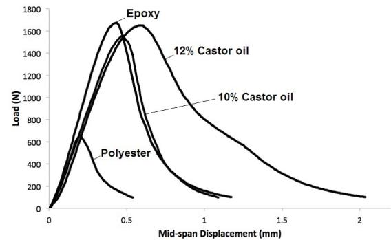
**Figure 4.** Typical load vs. mid-span displacement curves of castor oil and synthetic polymer mortars.
