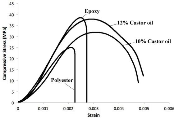
**Figure 1.** Typical compressive stress vs. strain of castor oil and synthetic polymer mortars.
