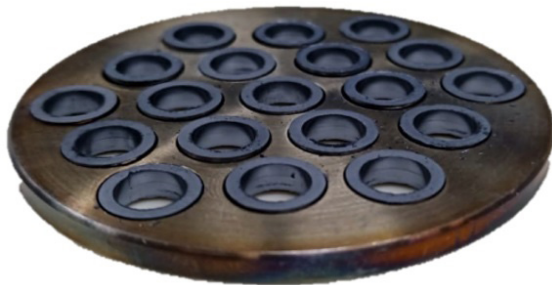
Figure 1. Cover configuration with cylinders for deposition.
