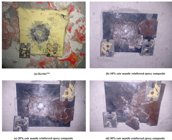
Figure 6. Aspect of MASs with different second layers after ballistic test against 7.62 mm bullet: (a) Kevlar™; (b) 10% coir mantle; (c) 20% coir mantle; and (d) 30% coir mantle reinforced epoxy composite.
