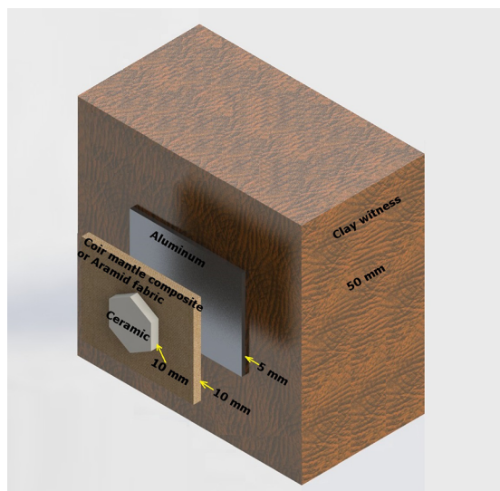
Figure 2. Schematic of the MAS placed in front of a block of clay witness simulating a human body.
