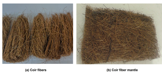
Figure 1. Coir fibers extracted from the mesocarp in the husk of a green coconut fruit (a) and coir fiber mantle (b).
