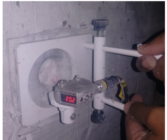
Figure 5. Measurement of the depth of indentation in the clay witness due to the remaining energy from the ballistic test 7.62 mm bullet impact against MAS.
