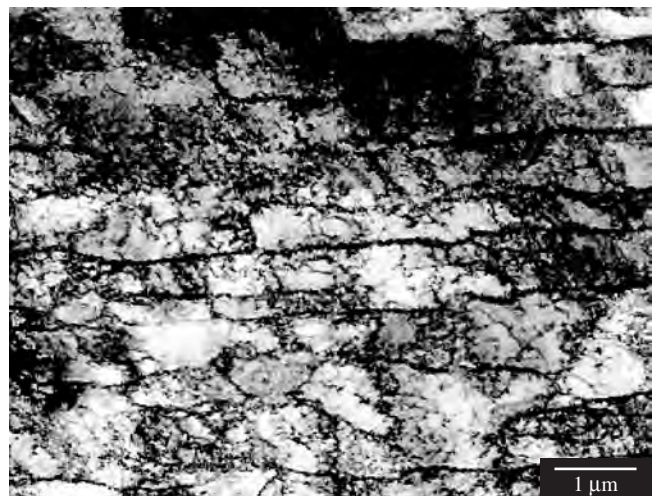
Figure 3. TEM of annealed steel submitted only to cyclic torsion (11.2% strain per cycle, 10 cycles).
