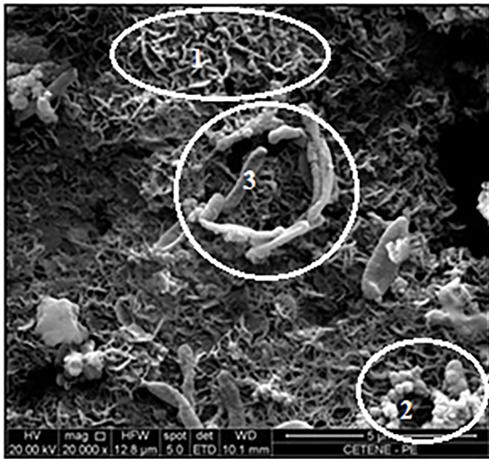
Figure 6. SEM of the specimen exposed in the water-containing region, immersed in oil/water system after 60 days; Magnification: 20.000X.
