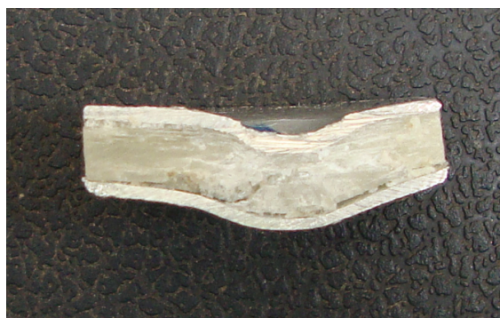
Figure 4. Photograph showing debonding of outer Al layer in UDHL (8.5 J).
