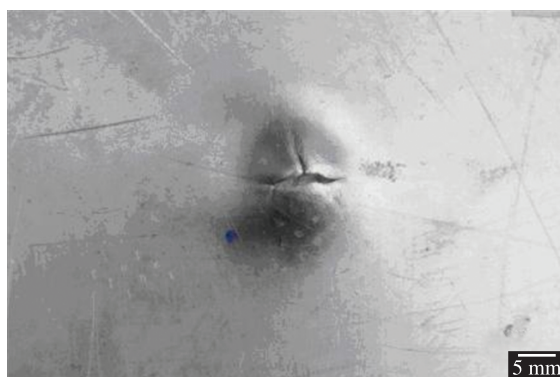
Figure 7. Crack initiation directions in CPHL.
