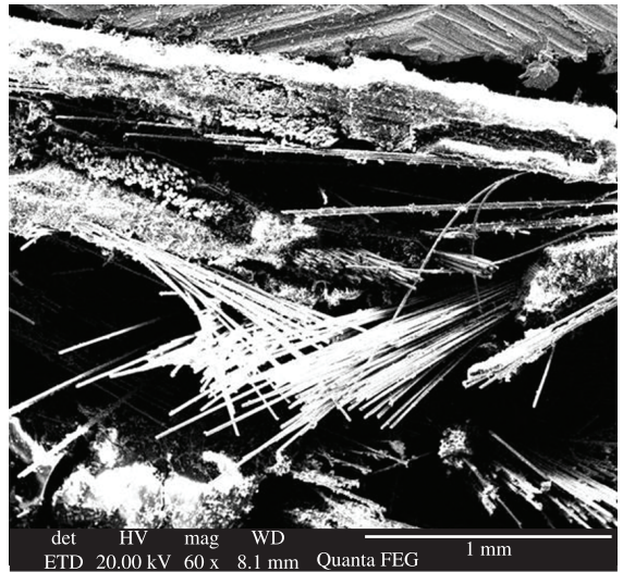
Figure 10. Extensive fiber breakage and matrix cracking at increased I.E. of 31 J in UDHL.
