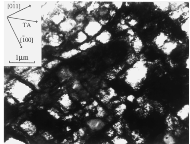
Figure 6. TEM observation of closed parallelogram cells developed near the rupture line during the second deformation in a grain with \langle 110 \rangle axis normal to the sheet plane. The prestrain value in rolling is equal to 0.16 (TA, tensile axis).
