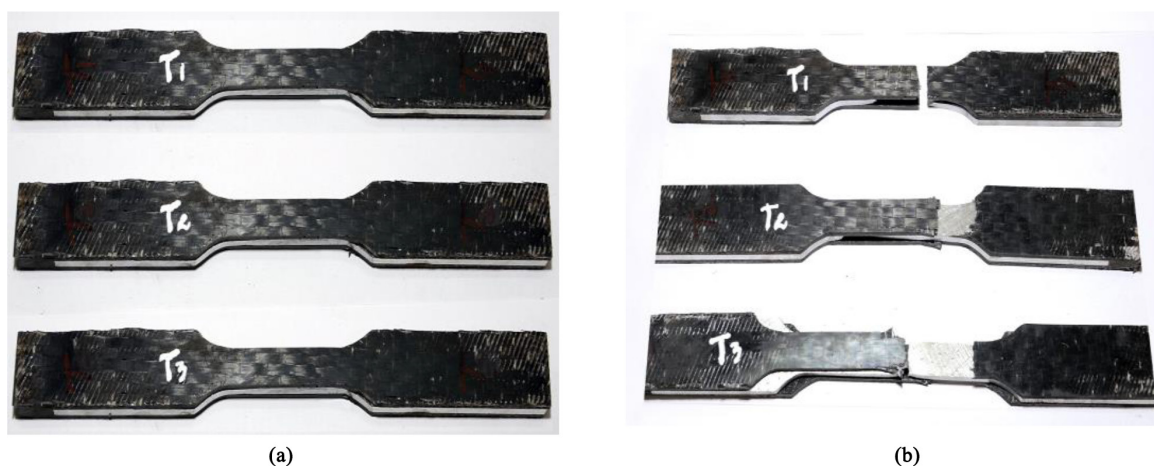
Figure 2. The specimen before tensile test (a), and after the fracture (b).
