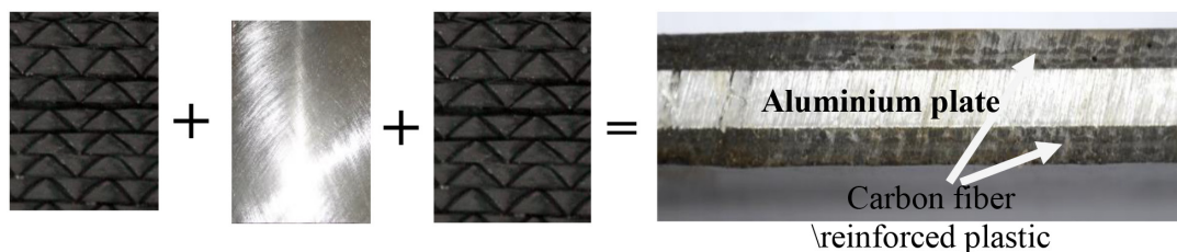
Figure 1. Schematic illustration of aluminium sandwich carbon fiber reinforced composites.
