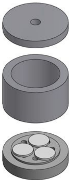
Figure 8. Arrangement of the sample holder with the cathode buttons.
