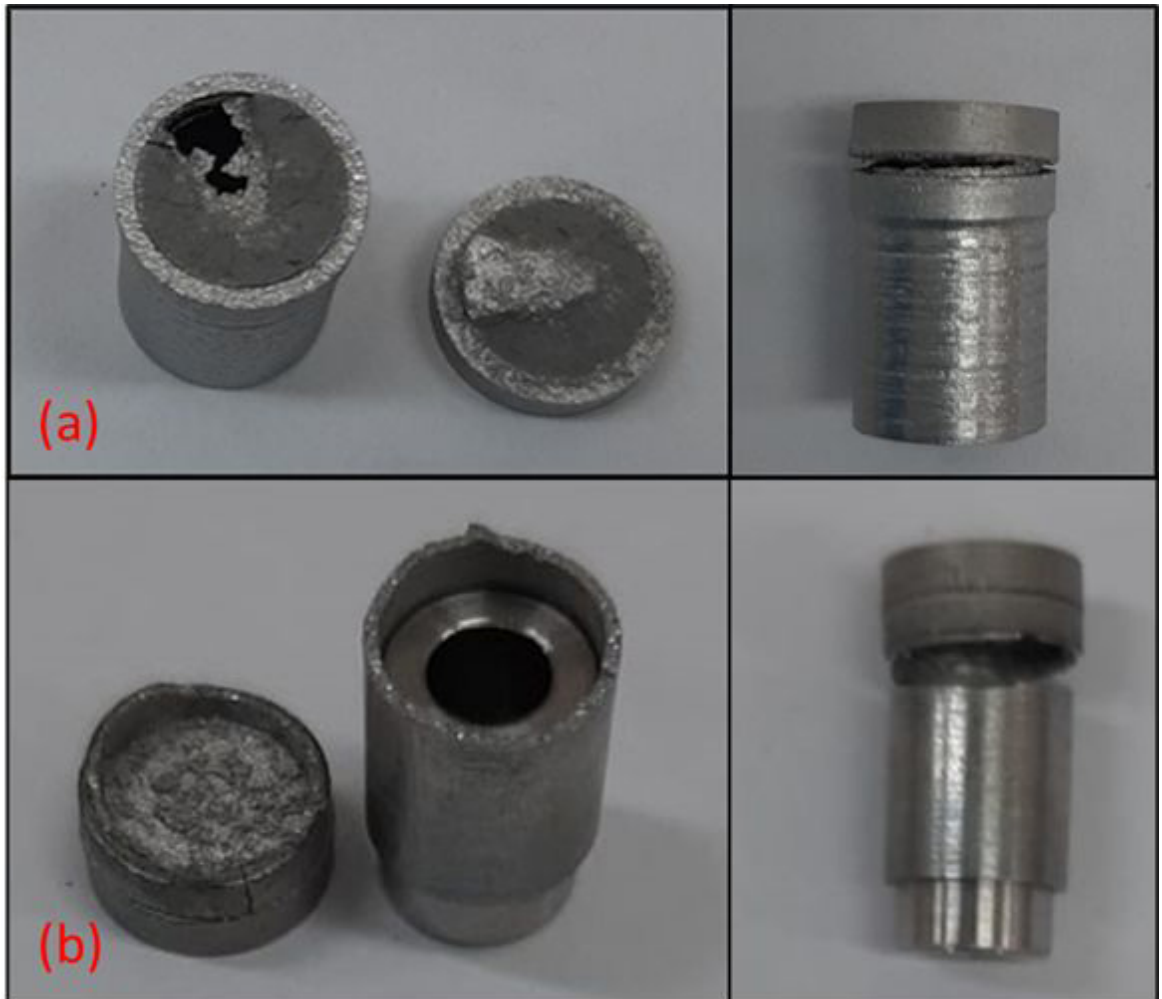
Figure 15. (a) cathode sample 1 after strength test, and (b) cathode sample 3 after strength test.
