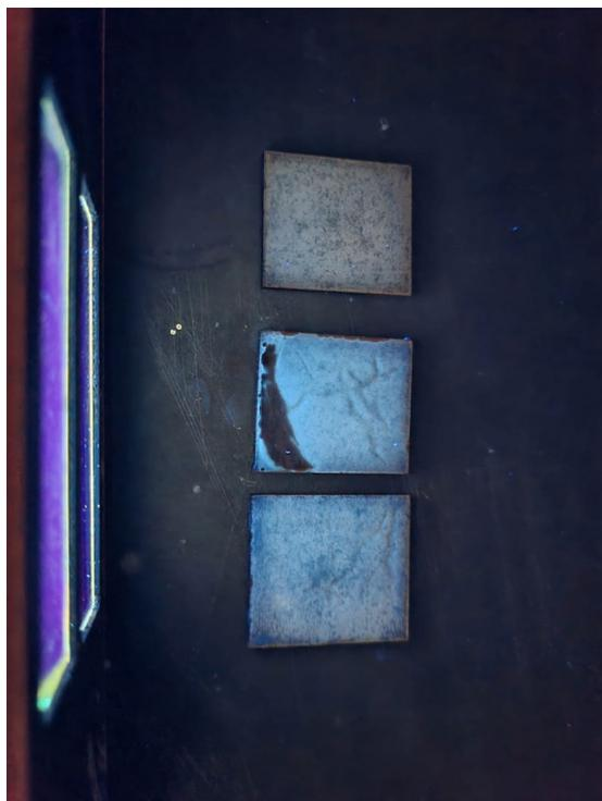
**Figure 7.** Test specimens without and with acrylic resina and CQDs coating under UV radiation.
