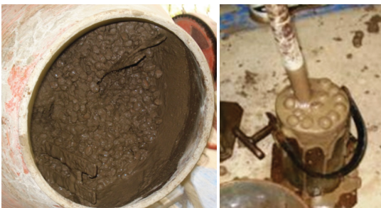
Figure 7. Concrete specimens preparation.
