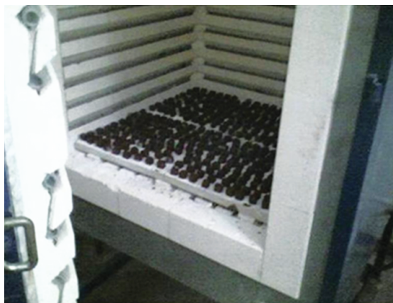
Figure 5. RM coarse aggregates sintering.
