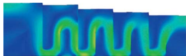
Fig. 2. Mean velocity distribution in the fish pass (see Fig.3 for legend).
