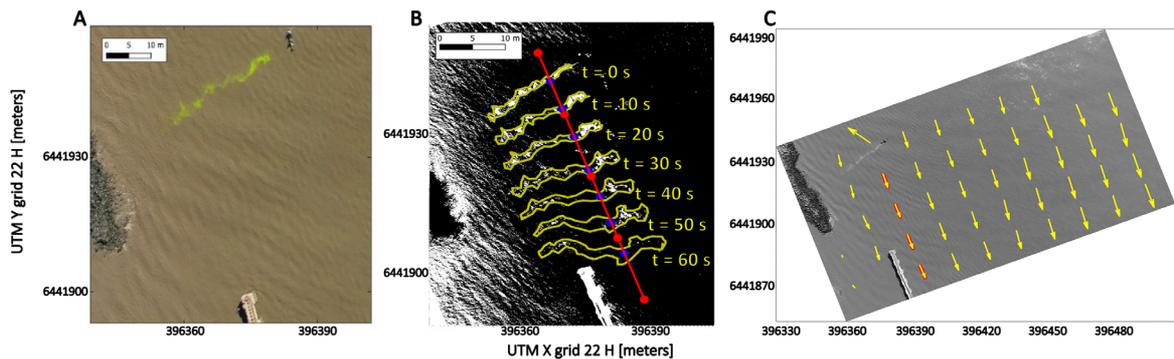
**Figure 2.** (a) snapshot from the drone immediately after the dye is released; (b) temporal evolution of the dye drift and scattering, the red dots indicate the drone vectors and the blue dots are the selected points in the dye; and (c) field of current velocity vectors generated after processing. The vectors marked with red indicate those used to compare with the drift data.
