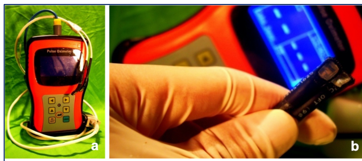
Figure 1. Pulse oximeter device adapted for Dentistry: (a) MD300A pulse oximeter model with "Y"-type sensor. (b) Diode sensors, one emitter of infrared light and the other receiver to measure pulp %SaO 2 (before PVC film protection).
