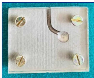
Figure 1. Cyclic fatigue testing device.
