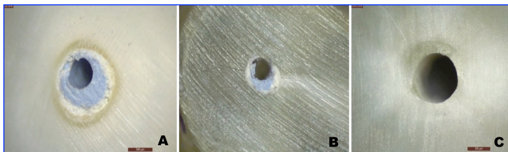
Figure 2. Stereomicroscopic images of the types of bond failure. (A) Cohesive failure, (B) Mixed failure, (C) Adhesive failure.
