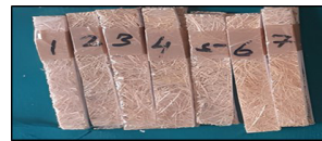
Figure 3. Various composition specimens for testing of impact strength of hybrid composites.
