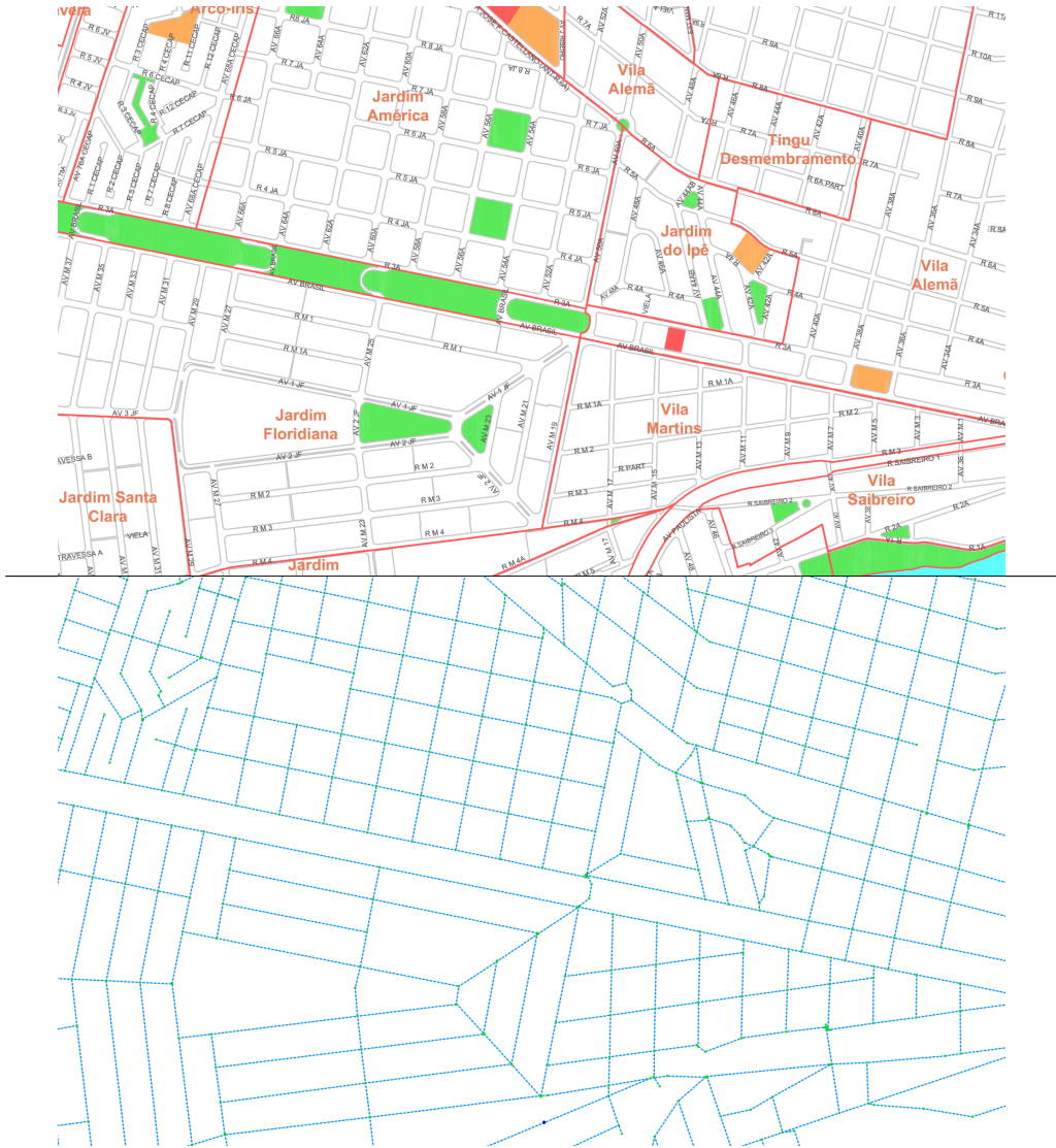
Figure 1 – Street modeling. Above a cropping of the original map and below the extracted streets (dashed in blue). The streets were extracted manually as a polygonal chain.
