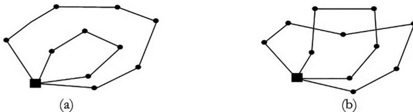
Figure 2 – a) Total and b) Partial Overlap between tow routes (Renaud, Boctor and Laporte, 1996[23]).
