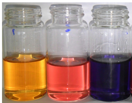
Figure 1. Color variation of solutions of 2 in solvents with decreasing polarity. From left to right: ethanol ( \lambda_{\max} 466 nm), 2-propanol ( \lambda_{\max} 494 nm), dimethylformamide ( \lambda_{\max} 587 nm)
