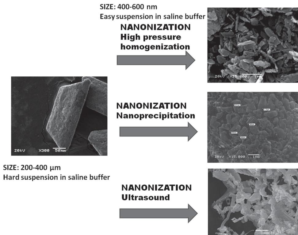
**Figure 6.** Scheme of nanonization (top-down processes) of P-MAPA
