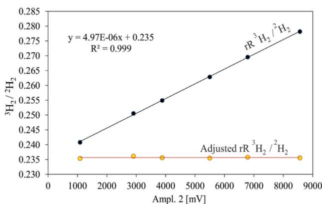
**Figure 2.** Graphic of  $^3\text{H}_2/{}^2\text{H}_2$  isotope ratio versus mass 2 signal amplitude for  $^3\text{H}$  Factor determination
