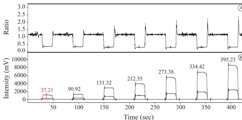
**Figure 1.** Typical values for  $^3\text{H}$  Factor determination. The graphic on top (A) shows the isotope ratio of masses 2 and 3 ( $3/2$ ) over time; bottom graphic (B) shows the intensity (mV) of mass 2 and 3 signals over time varying the pressure of the reference gas  $\text{H}_2$ , with the upper plateau being mass 2 and bottom plateau mass 3
