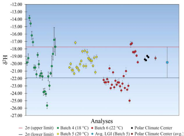
**Figure 4.** Diagram of  $\delta^2\text{H}$  values versus the number of analyses in the LGI control sample - control chart
