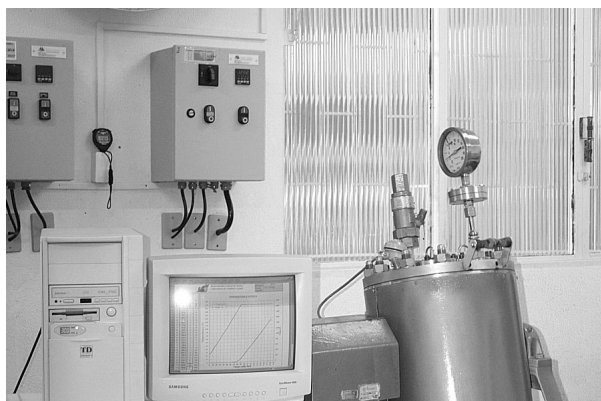
Figura 1 – Digestor Batch computadorizado, com quatro reatores. Figure 1 – Computerized batch digester, four reactors.
