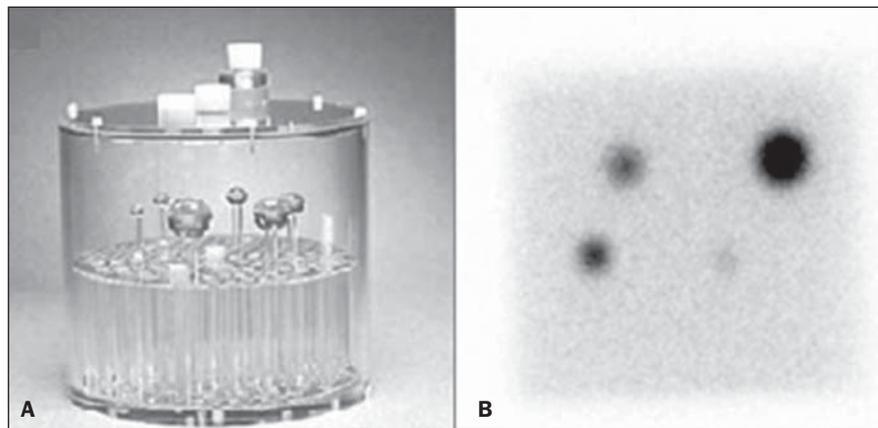
**Figure 1.** Image of the Jaszczak phantom utilized in the experiment (A) and lateral view showing the spheres positioning (B).
