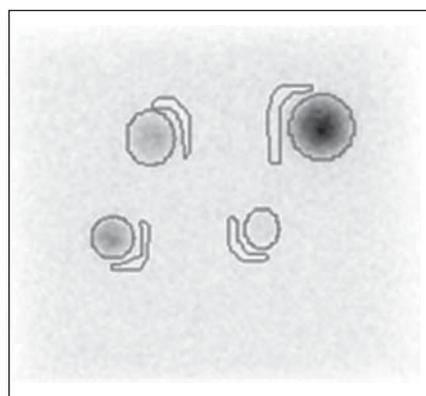
**Figure 2.** Examples of ROIs selected over spherical sources and selected regions for background subtraction.
