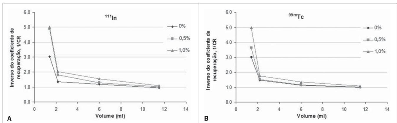
**Figure 3.** Curves of the recovery coefficients reverse (1/RC) determined for <sup>111</sup>In (A) and <sup>99m</sup>Tc (B) as a function of sphere volume.
