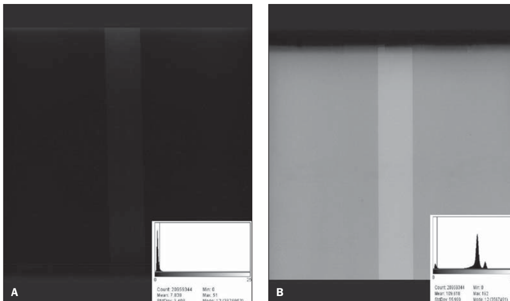
Figure 1. Comparison between images from the analog system for 117 kVp and 4 mAs exposure factors from the Siemens equipment (high frequency) (A) and from the Emic equipment (12 pulse) (B).
