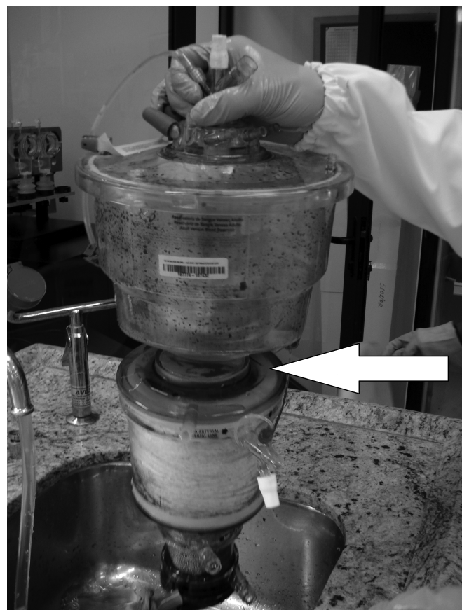
Figure 1 – Oxygenator and Venous Reservoir. The Arrow Indicates the Site of the Crack.
