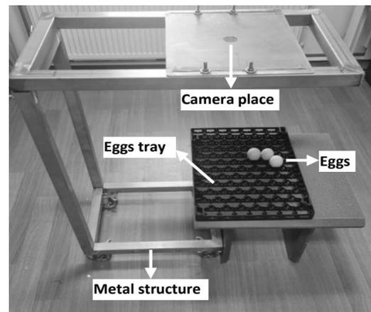
Figure 2 – Hatchery image acquisition system (Tekin, 2023).
