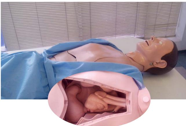
Fig. 5 - Dummy with removable chest wall. Highlighted, view from inside the chest cavity molds with viscera of the chest and upper abdomen.
