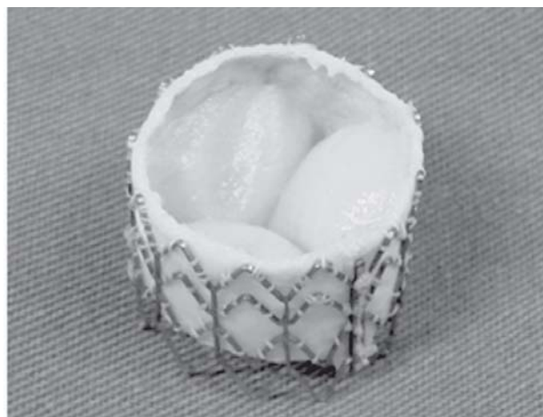
Fig. 1 – Final model of aortic bioprosthesis for mounting on balloon catheter
