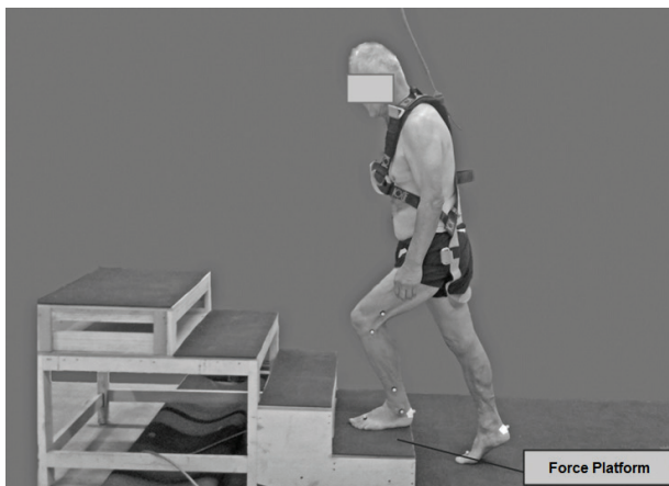
Figure 1. Position of the force platform in the stairs and a participant using the safety harness.
