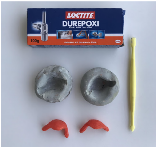
Figure 3. Silicone cartilages and the material for their manufacture.
