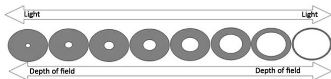
Figure 2. Simplified diagrammatic representation of the diaphragm (set of superimposed blades— “leaf shutter”—inside the lens that allows control of the amount of light entering the camera). The diaphragm aperture values are indicated by “f” (in the diagram, from left to right: f/16, f/11, f/8, f/5.6, f/4, f/2.8 and f/1.4). The larger the number, the more closed the diaphragm, and therefore less light will pass through the hole. The aperture of the diaphragm also controls the depth of field (extension of the sharp region [in focus] when taking a picture); the greater the aperture of the diaphragm (i.e., the smaller the number), the smaller the depth of field. In medical photos, maximum clarity of the subject/patient is sought so that details are not lost; this is achieved by adopting small diaphragm apertures, preferably > f8. Note: The proportions of distances and sizes in the sketch are not true-to-life.
