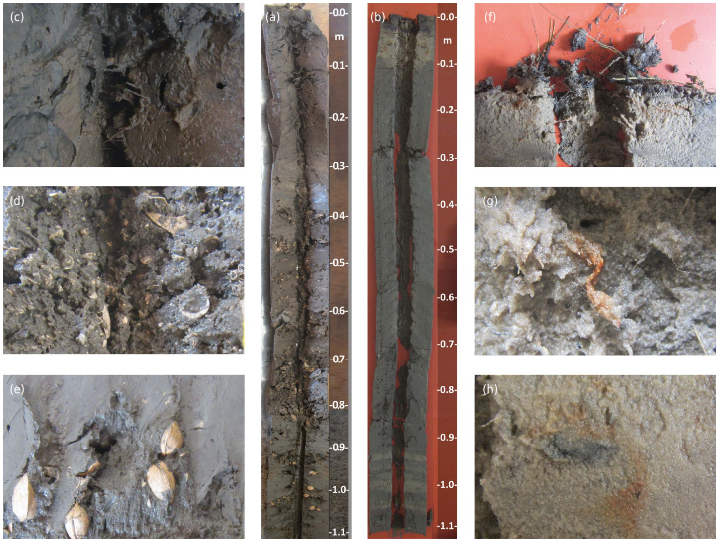
Figure 3. Subaqueous soil profile of the semiarid coast in the Northeast (a) and the Quaternary coast in the South of Brazil (b). In details, the variegated colors of the Agj horizon (0.00-0.10 m) (c); broken seashells within a sandy texture matrix (2Cgjz horizon; 0.56-0.84 m) (d); whole seashells within a clayey matrix (horizon 3Cgjnz, 0.84-1.14 + m) (e), from the NE semiarid coast; surface soil horizon Agj (0.00-0.06 m) (f); mottles from sulfide production (black) and iron oxidation (brown) (ACgj horizon, 0.06-0.13 m) (g), and rhizospheric oxidation resulting in Fe oxyhydroxide precipitation (ACgj horizon, 0.06-0.13 m) (h) from the Quaternary coast in the South.
