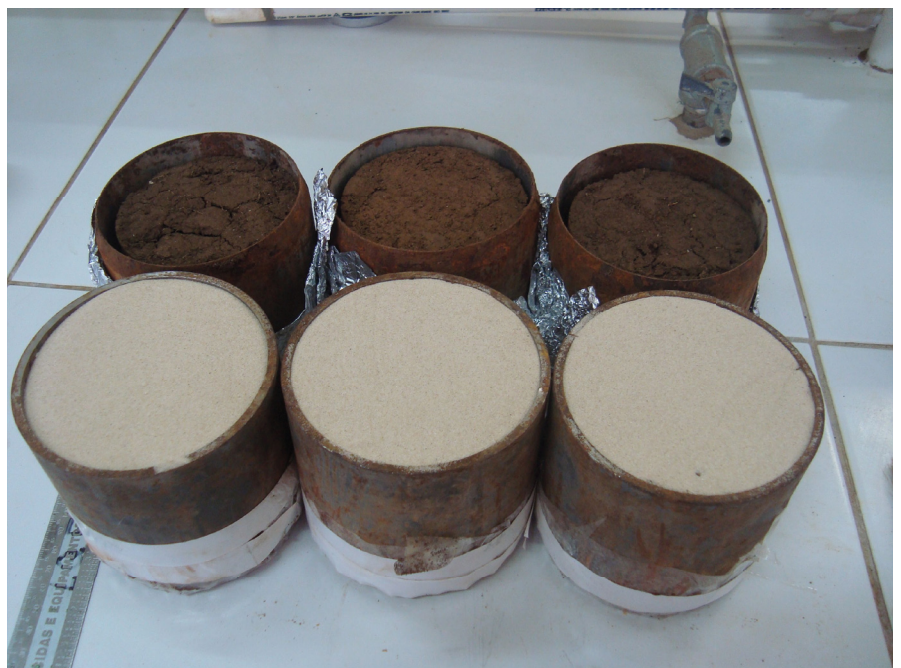
Figure 2. Volumetric rings with soil mass shrunken and after filling with sand (Ring with Sand Method).
