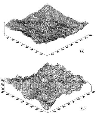
Figure 2. Three-dimensional representation of the soil profile before (a) and after tillage (b), assessed by a laser profile meter (in cm).
