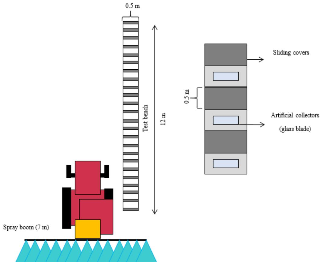
The wind direction was maintained in the range of 0- 40° on the test bench
