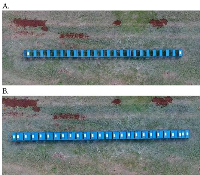
**Figure 2.** Test benches with all collectors covered, except for the first and last, for the entire duration (A), and test benches with collectors uncovered (opened) to collect spray (B)
