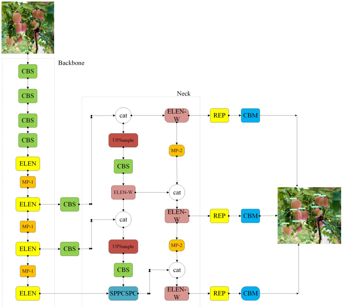
Figure 2. Structure diagram of the YOLOV7 visual recognition network
